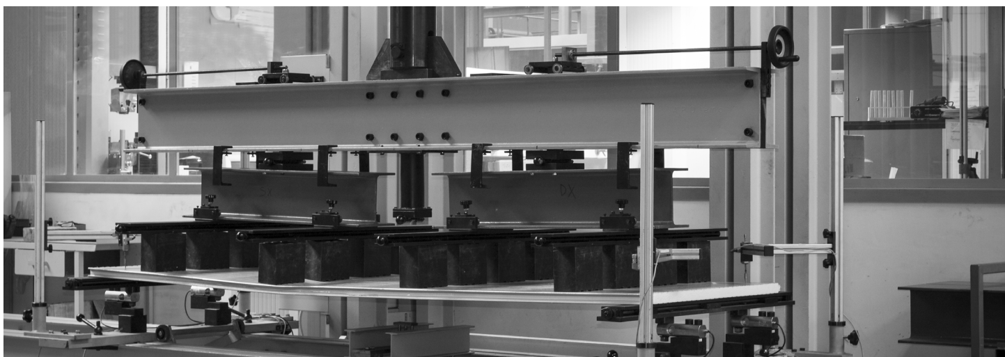
Picture n° 6: bending tests on wall panel at Isolpack's laboratory / Vinovo plant (TO)
